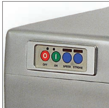
Simple electronic control panel for semi-automatic operation.
